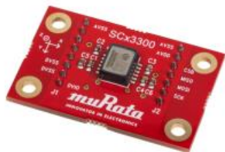
Murata 3-axis accelerometer SCA3300-D01
