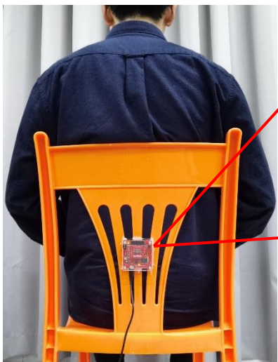
Murata 3-axis accelerometer SCA3300-D01
