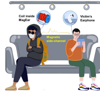
Figure 1: Illustration of MagEar. The adversary disguised MagEar as headphones to eavesdrop on a victim.
