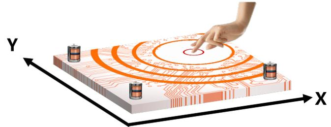
Fig. 1: MM-Tap can localize finger tap on ubiquitous surfaces with three geophone sensors.
